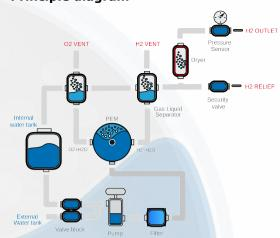
Hydrogen is produced from distilled water using a polymeric membrane (PEM). No acid or alkaline solutions are used.
